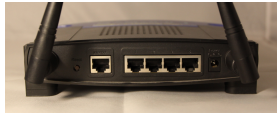
The two pictures below show a Linksys WRT54GL Wireless-G Wireless Router with a WAN port and a 4-port switch
