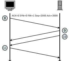
3. The diagram shows the termination of a TCP connection. Complete the table.
