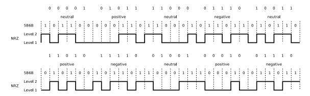
4. These signal curves are encoded with NRZI and 4B5B. Decode the data.
